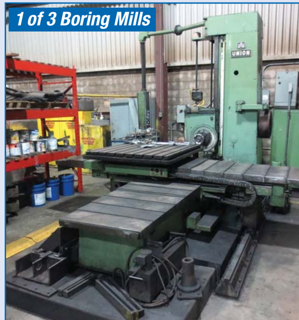
UNION 4" Horizontal Boring Mill, Model BFT-102
